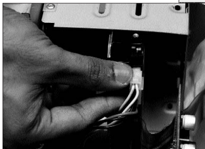
Finally connect the power cable to the hard drive
